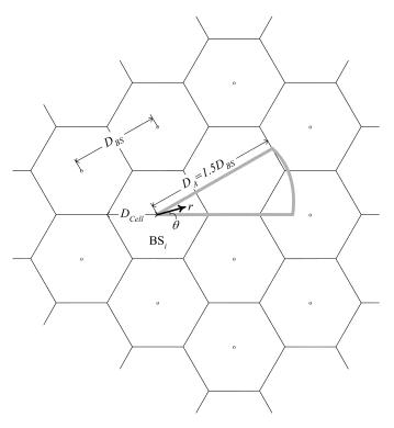
Fig. 2. Cell sites deployment model.
