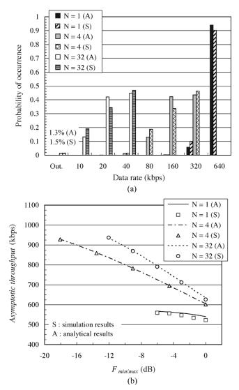
Fig. 9. Comparison of analytical results and simulation results: Rate Set I. (a) The pmf of the assigned data rate. (b) Tradeoff between throughput and fairness.
