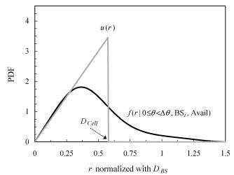
Fig. 3. Distribution of the connected user to a BS.
