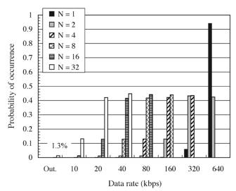
Fig. 5. The pmf of the assigned data rate: Rate Set I.
