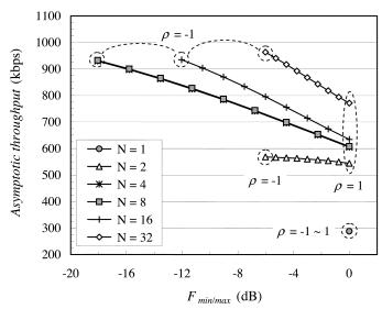
Fig. 11. Tradeoff between throughput and fairness: Rate Set II.
