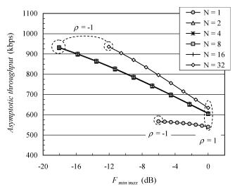
Fig. 8. Tradeoff between throughput and fairness: Rate Set I.
