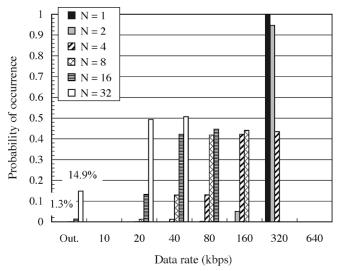
Fig. 10. The pmf of the assigned data rate: Rate Set II.
